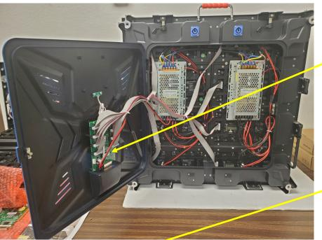
First Always Disconnect the 2 CAT5 so the Cabinet can enter in TEST mode, on the controller board there's a TEST button, press several times until the Screen is WHITE.
